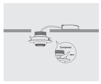
2. Compress spring plates and insert into cutout hole.
